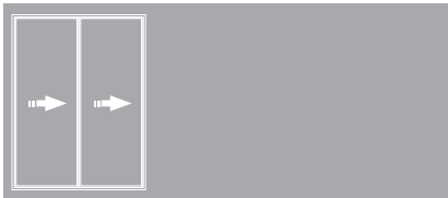
TWO PANE CONFIGURATION (2 panes, 2 sliding, 0 swing)
